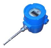
Desinged for inexpensive Non-hazordous use Low power dissipation, under 2.5 Watts (e.g., under 100 ma at 24 VDC) Accuracy (and linearity) : ±[1% of Reading +(.5% FS)] Integral and remote styles 24 VDC or 115VAC/230 VAC Flow Rate, Totalizer 4 to 20 mA for Rate; 24VDC pulse for Totalized value RS232 Communication Modbus® compliant RS485 RTU communications (optional) Field reconfigurability via optional Addresser software
